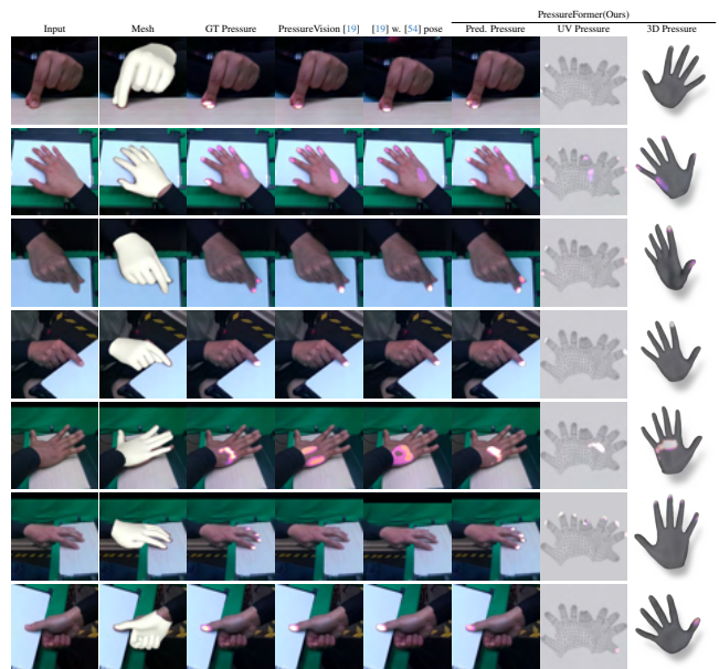
Figure 11. Qualitative Results PressureFormer on our dataset. We compare our PressureFormer with both PressureVisionNet [19] and our extended baseline model with HaMeR-estimated [54] 2.5D joint positions. Additionally, we provide visualizations of the hand mesh estimated by HaMeR, alongside the 3D pressure distribution on the hand surface derived from our predicted UV-pressure in the last two columns. Note that we transform the left-hand UV maps into the right-hand format.
