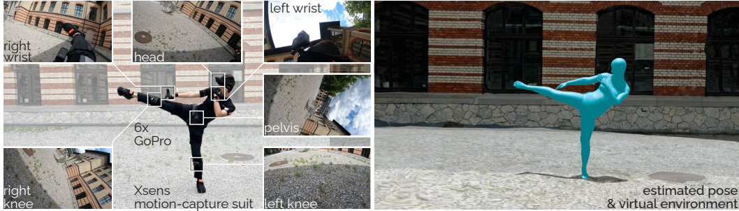
Figure 1: (Left) Our dataset MultiEgoView contains 5 hours of egocentric real-world footage from 6 body-worn GoPro cameras and ground-truth 3D body poses from an Xsens motion capture suit as well as 119 hours of simulated footage in high-fidelity virtual environments on the basis of real motion capture data and associated 3D body poses. (Right) Our method estimates ego poses from video data alone, here visualized inside the scanned 3D scene.
